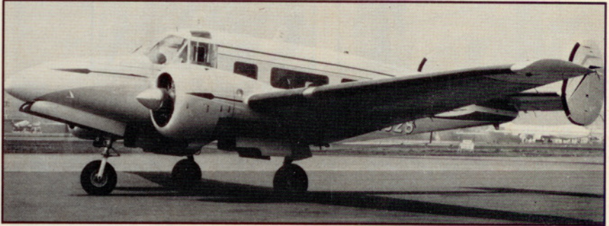
Beech's final production Model 18 was the Super H-18, which featured tricycle landing gear.
