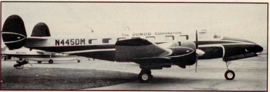
The Dumod Corporation stretched the Model 18 to 43 feet five inches, producing a 15-seat airliner.
